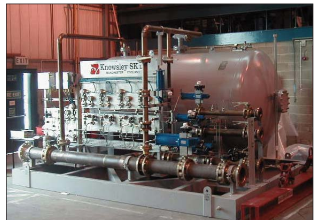
Figure 4. Bladder tank construction at the KSK workshop
